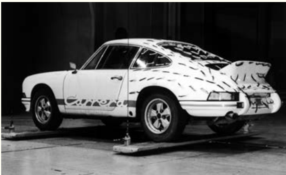
above – Early windtunnel tests right – The Geneva Motor Show in 1973
