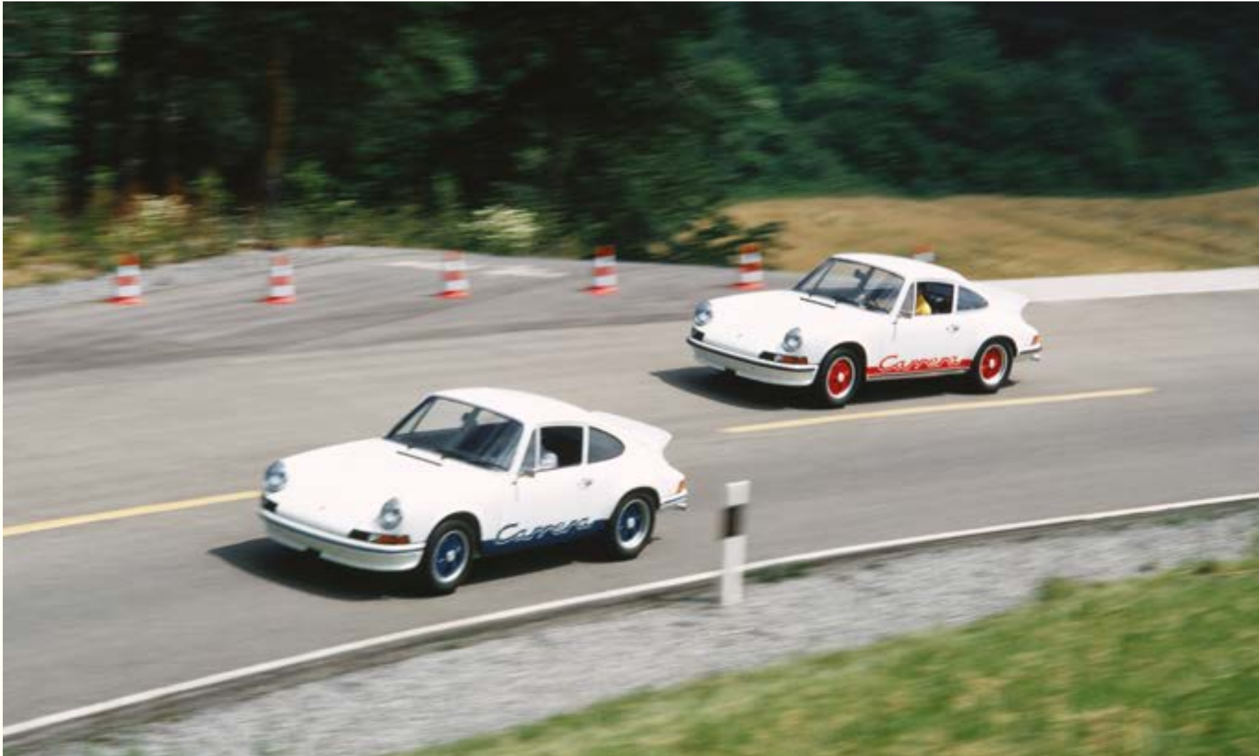
A publicity shot showing prototype cars with the front spoiler of the 911 2.4 S instead of the real 2.7 RS front spoiler. The one with the blue striping is a lightweight prototype, the one with the red striping is a touring prototype.
